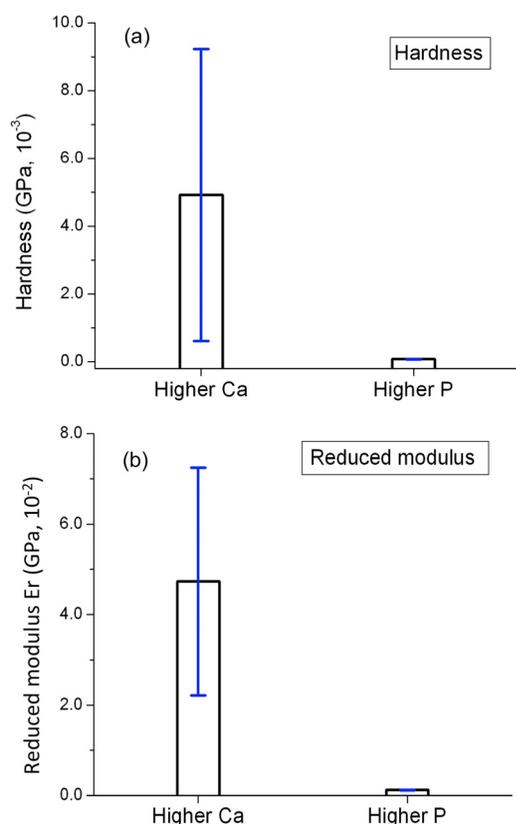
FIG. 3. (Color online) Variations in the hardness (a) and reduced modulus (b) of the nanocomposite scaffolds prepared with higher calcium (Ca) and higher phosphorous (P).
