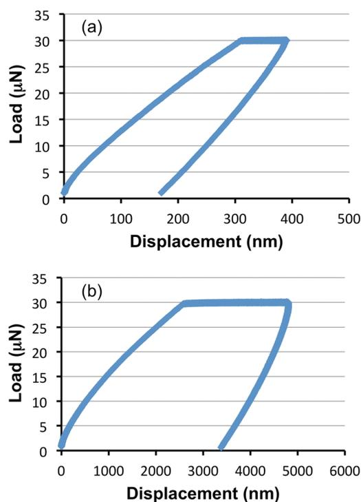
FIG. 2. (Color online) Typical graphs of the load vs. indentation depth for the bionanocomposite scaffold in the case of (a) higher calcium mineralized and (b) higher phosphorous (and HAP) mineralized.
